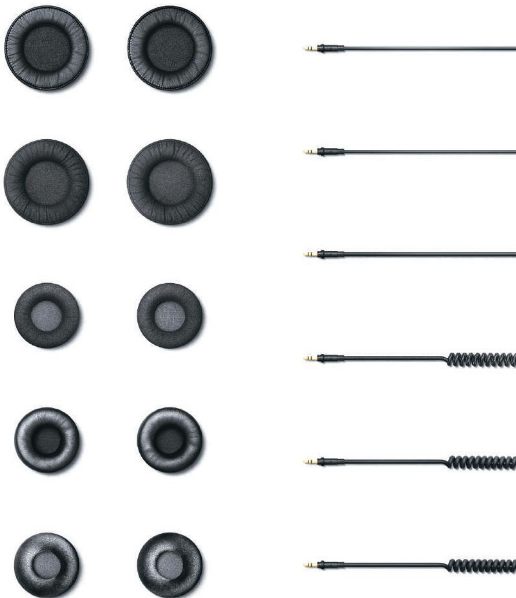
Photo: The TMA-2 Modular Headphone from the Danish headphone manufacturer AIAIAI is designed as a framework of elements, including the speaker unit, headband, ear pads and cable, which can be connected or combined in different ways. 17 The parts are bought and assembled according to the specific requests of the user, which allows for mass customization. The design also allows for disassembly of the headphones if the customer are to upgrade certain parts or change them if something breaks. 18
