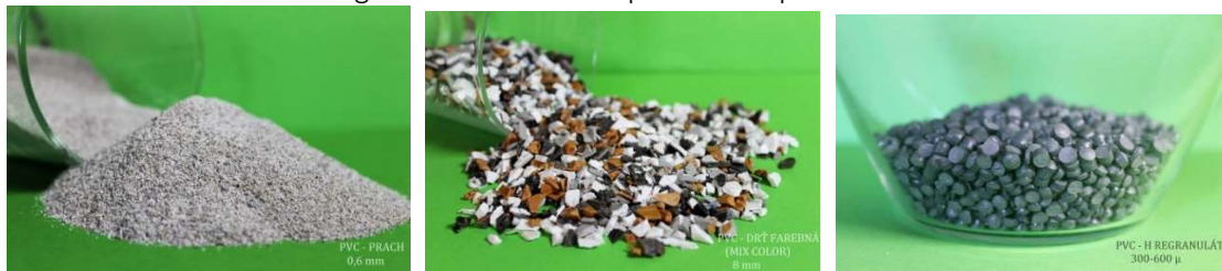
Figure 12 Recycled PVC dust, chips and granulate
